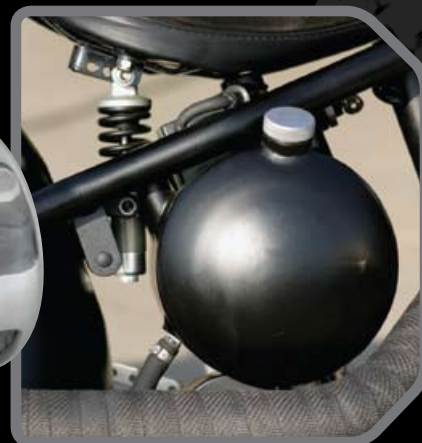
Oilbag with electric-start clearance - rear view
